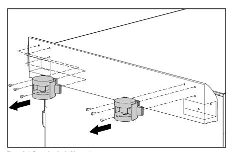
Figure 2-1. Removing the locking casters
